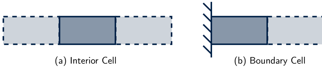
Figure 11: A comparison of interior cells (a) and boundary cells (b) in the mesh.
